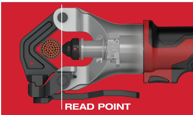
Auto Distance Control combined with continuous pressure monitoring enables the tool to sense the instant it contacts the connector; analyzing the outside diameter of the connector to determine its size, and simultaneously setting a target final crimp distance.
